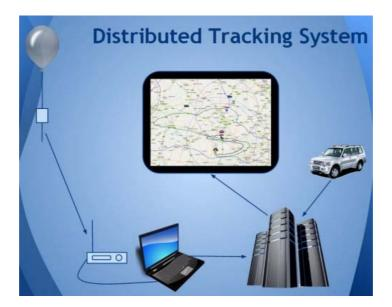
The above shows how the UKHAS system works. Your balloon carries a radio tracker that sends its position (and perhaps sensor data, or even images) down to the ground, where it is received by one or more listening stations. **I**
