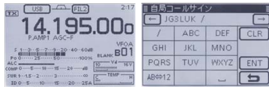
Tap C Showing Multi-Function Meter
